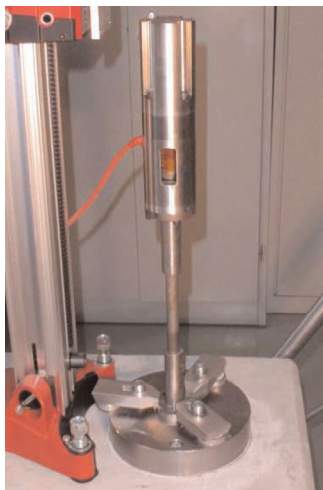
Figure 5: Symmetrical pulse generator vertical arrangement. Both sides are coupled to steel bars for two-sided impulse extraction. Notice the casing and mounting flanges steel for getting optical access for the LDA-measurements.
